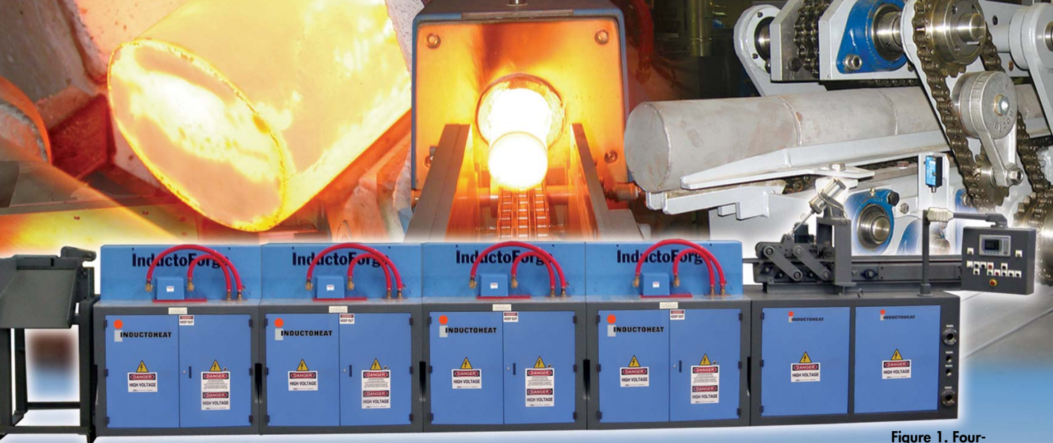
Figure 1. Four-module InductoForge progressive, horizontal induction billet heater
